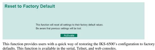
**NOTE** After restoring the factory default configuration, you will need to use the default network settings to re-establish the web or Telnet console connection with the IKS-6500.
