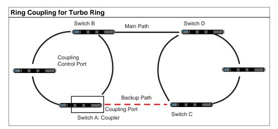
To configure the ring coupling for a **Turbo Ring**, select two IKS series Ethernet switches (e.g., Switch A and B in the above figure) in the ring, and another two IKS series Ethernet switches in the adjacent ring (e.g., Switch C and D).
