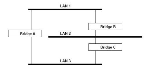
If STP is enabled, it will detect duplicate paths and prevent, or block, one of them from forwarding traffic. In the following example, STP determined that traffic from LAN segment 2 to LAN segment 1 should flow through Bridges C and A because this path has a greater bandwidth and is therefore more efficient.
