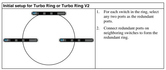
The user does not need to manually assign the master with Turbo Ring or Turbo Ring V2. If no switch is assigned as the master, the protocol automatically selects one of the switches to be the master. The master is only used to identify which segment in the redundant ring acts as the backup path. In the following subsections, we explain how the redundant path is selected for rings configured for Turbo Ring and Turbo Ring V2.
